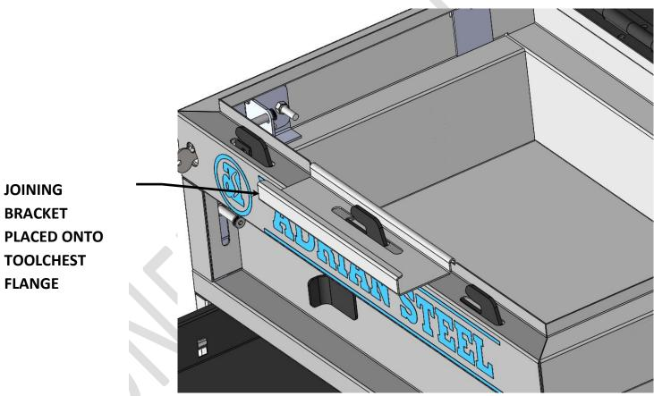
**BRACKET PLACED ONTO TOOLCHEST FLANGE**
