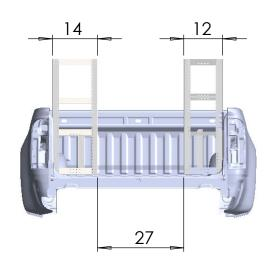
**CAUTION:** DRILL THRU FLOOR WITH CARE! WATCH FOR GAS TANK, CONTROL LINES, & ELECTRICAL WIRING.
