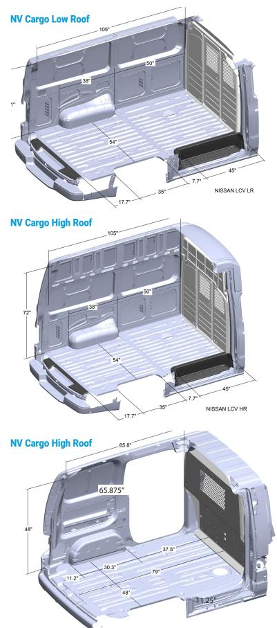
\* Subtract 3" from dimension when a Max Comfort partition wing kit is installed. Note: Dimensions for reference only. Measure your van or contact your distributor for your exact needs.
