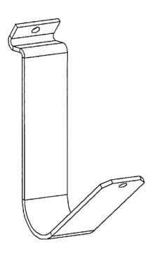
NOTE: SUSPENDED LOAD PER Z-RAIL HOOK SHOULD NOT EXCEED10 LBS.
