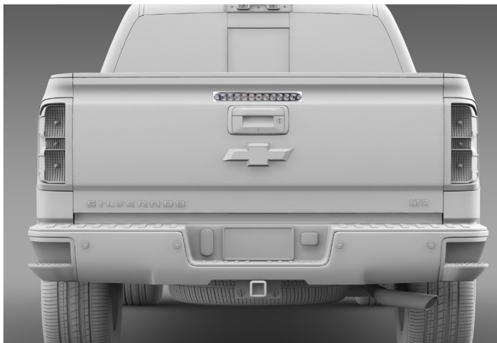
CHMSL Circuit OEM Wire. Brown/Yellow Wire
