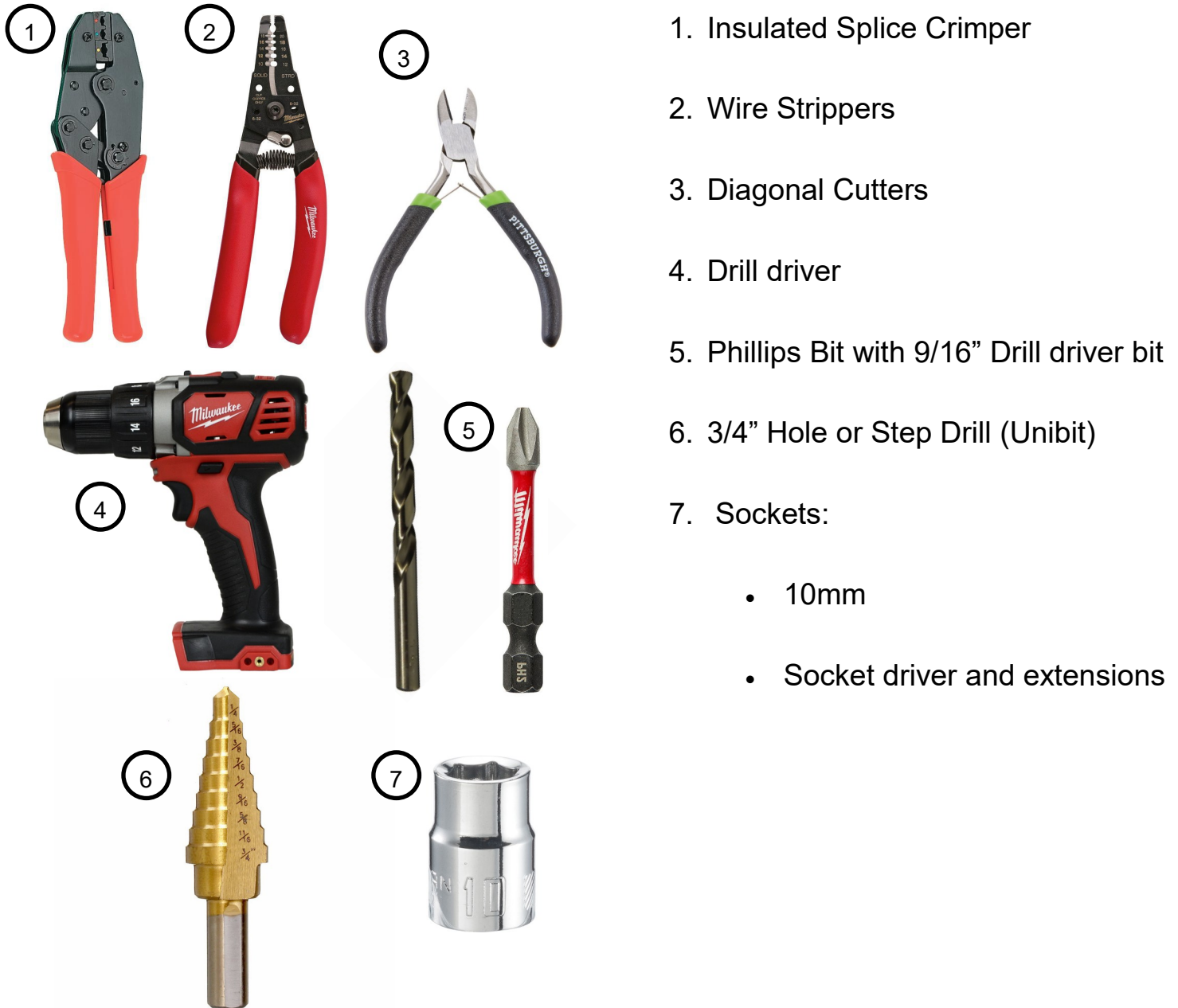
Figure 4-1: Tools Needed for Installation
