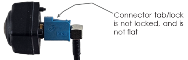
Not Fully Seated Connection
