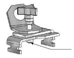
Thread hand knob into part until it just extends slightly out the bottom as shown. (The exact amount is not important right now)
