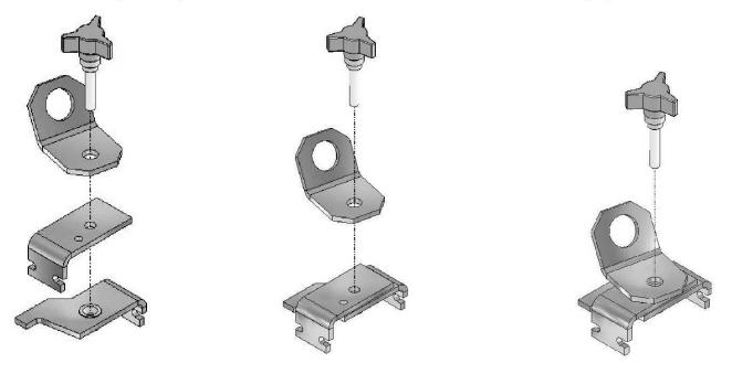
Partially thread hand knob into lock retainer (bottom part) so the threaded portion extends just below the retainer plate.
