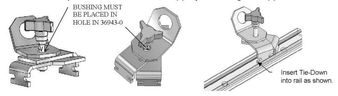
Once the parts are inserted into the rail, straighten the parts out as shown below.
