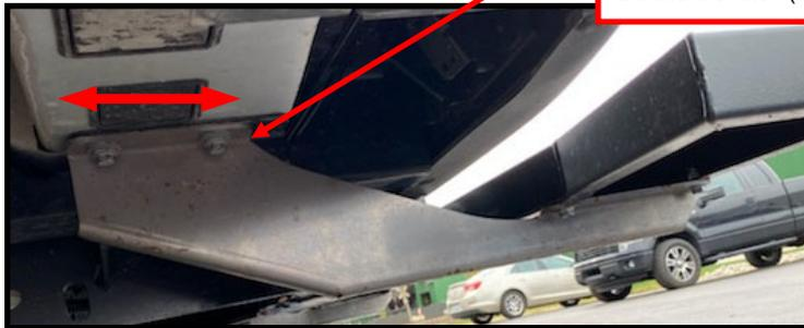
**Step 02** Loosely fasten the step body to the arms in four places as shown below. Leave loose for adjustment.
