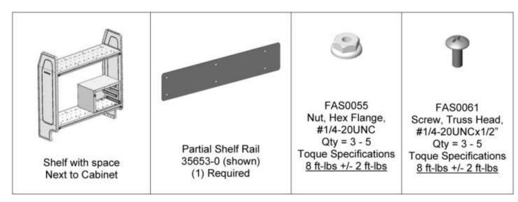
Attach Shelf Rail with Screws, placing nuts on back side. Torque fasteners as specified.
