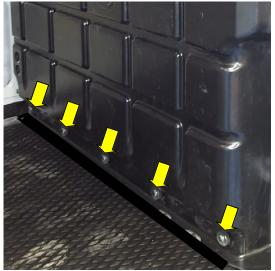
ATTACH THE PARTITION PANEL TO THE PARTITION FOOTER USING THE ABOVE LISTED 5/16" FASTENERS AT FIVE (5) PLACES AS SHOWN. FULLY TIGHTEN THESE FIVE (5) FASTENERS.
