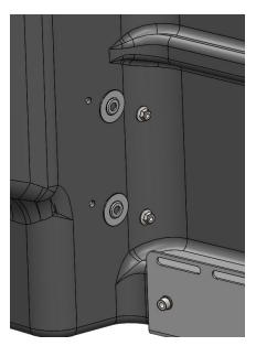
DETERMINE MOUNTING POSITION FOR ACCESSORY AND MARK HOLE LOCATION(S). DRILL 5/16" DIAMETER HOLES THRU PARTITION PANEL. USE 1/4" TRUSS HEAD SCREWS THRU THE ACCESSORY WITH CUP WASHERS FROM THE CAB SIDE OF THE PARTITION AND USE NYLOCK FLANGE NUTS TO SECURE ACCESSORY.
