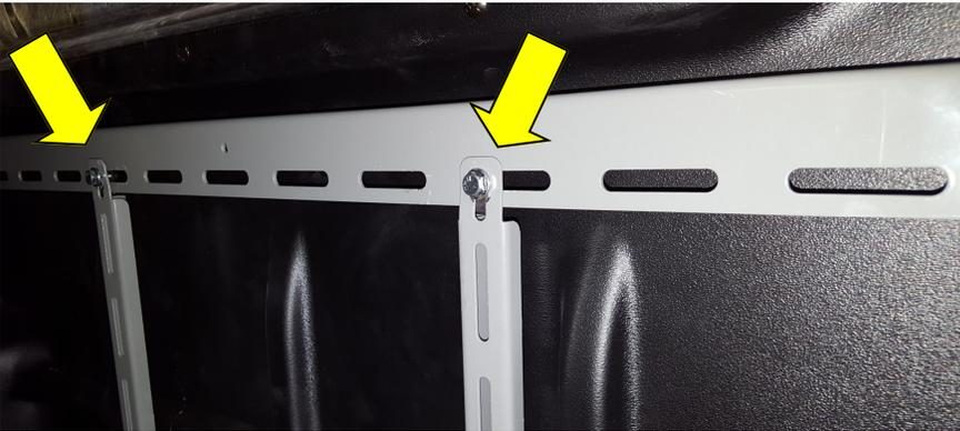
ATTACH TWO SPRING CLIPS TO THE CROSS CHANNEL IN THE 5TH AND 10TH SLOTS WITH THREADED PORTION FACING TOWARDS THE REAR OF THE VEHICLE AS SHOWN.
