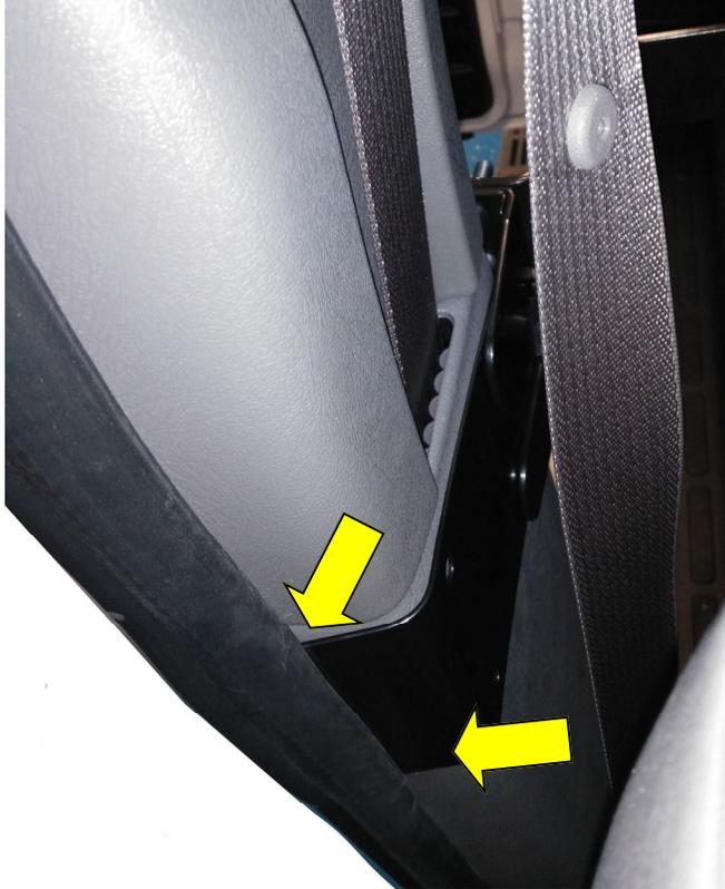
RE-ATTACH DOOR SEALS ONTO THE B-PILLAR FLANGES AND OVER THE B-PILLAR BRACKET HEMMED EDGES.
