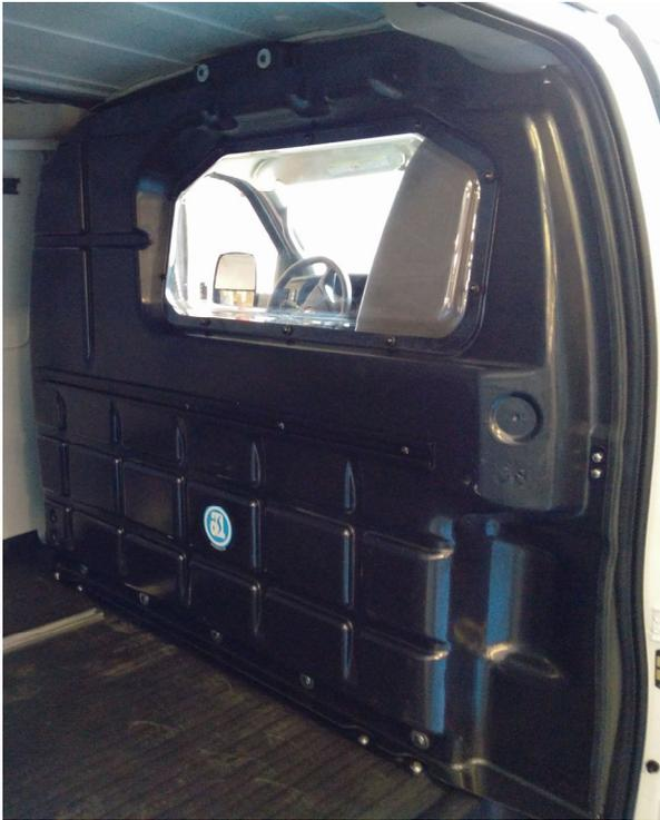
INSERT PARTITION INTO VEHICLE WITH BOTTOM EDGE WAY FROM THE FOOTER WITH THE TOP CONTACTING THE HEADER AREA FIRST AND THEN PIVOT UP AND FORWARD INTO PLACE AGAINST B-PILLARS AND FOOTER.
