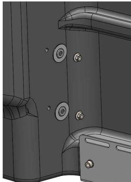
DETERMINE MOUNTING POSITION FOR ACCESSORY AND MARK HOLE LOCATION(S). DRILL 5/16" DIAMETER HOLES THRU PARTITION PANEL. USE 1/4" TRUSS HEAD SCREWS THRU THE ACCESSORY WITH CUP WASHERS FROM THE CAB SIDE OF THE PARTITION AND USE NYLOCK FLANGE NUTS TO SECURE ACCESSORY.
