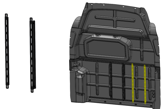
PARFTCAB (shown below in yellow) Cab side hardware mounting kit installed
