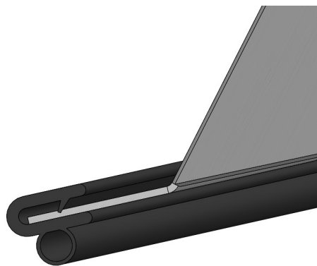
VIEW OF SEAL ON PARTITION WING. BULB TOWARD FRONT.
