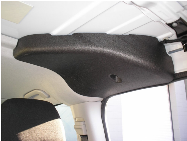
FOAM PAD, PASS SIDE REMOVE SCREW AND PULL OUT FROM ABOVE HEADLINER
