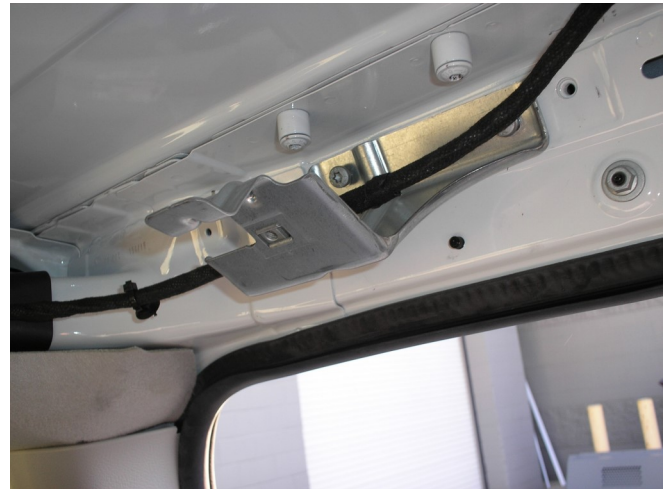
FOAM PAD REMOVED. NOW REMOVE BRACKET.
