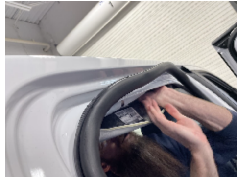
REACH UNDER THE HEADLINER AND SECURE (1) FAS0274 TO EACH GRAB HANDLE MOUNTING HOLE
