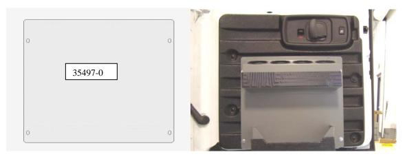
Open Vehicle rear door. Place AGWBHACT4 below latch handle on Curbside / passenger side. Center the unit between plastic liner hold down clips. Mark all four mounting locations using back plate as a jig. Make sure the bottom edge of the back panel is slightly above the bottom edge of the plastic liner. Otherwise it may interfere with the closing of the rear door.
