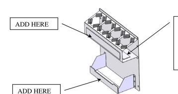
TAKE THE 26650-0 FOAM ROLLS AND ATTACH AS SHOWN. THIS IS FOR SOUND DEADENING PURPOSES AND SINCE THE AGWBHACT4 IS MOUNTED TO THE REAR DOOR, IT MAY COME IN CONTACT WITH A WINDSHIELD THAT IS IN THE AUTO GLASS RACK WHEN THE REAR DOOR IS CLOSED.
