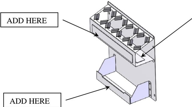
TAKE THE 26650-0 FOAM ROLLS AND ATTACH AS SHOWN. THIS IS FOR SOUND DEADENING PURPOSES AND SINCE THE AGWBHACT4 IS MOUNTED TO THE REAR DOOR, IT MAY COME IN CONTACT WITH A WINDSHIELD THAT IS IN THE AUTO GLASS RACK WHEN THE REAR DOOR IS CLOSED.
