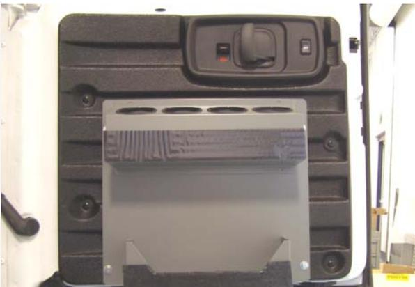
Open Vehicle rear door. Place AGWBHACT4 below latch handle on Curbside / passenger side. Center the unit between plastic liner hold down clips. Mark all four mounting locations using back plate as a jig. Make sure the bottom edge of the back panel is slightly above the bottom edge of the plastic liner. Otherwise it may interfere with the closing of the rear door.
