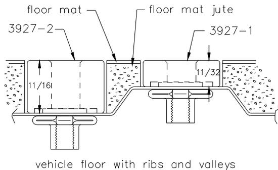
The location of various floor mounts will determine what spacer combination will be used. For example, an 11/32" spacer is used atop floor ribs, and an 11/16" high spacer is used atop floor valleys.
