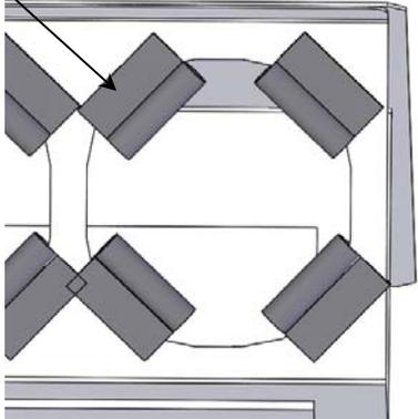
**The foam inserts need to be installed on the inside with the flat washers next to the foam. Be careful not to over tighten the fasteners when installing the foam inserts.**
