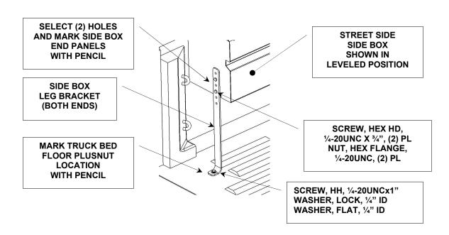
Position the SIDEBOX TIE BRACKET as shown, mark all (4) through holes on the crossbox and side box panels. Center punch all (4) holes and drill a 9/32" diameter hole, deburr holes as required.
