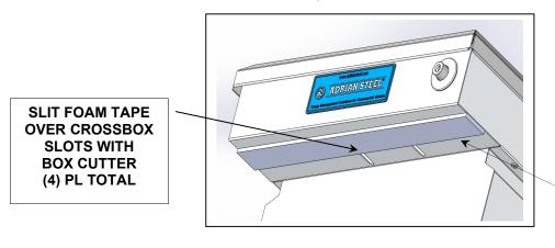
20" FOAM TAPE APPLIED TO CROSS BOX AS SHOWN
