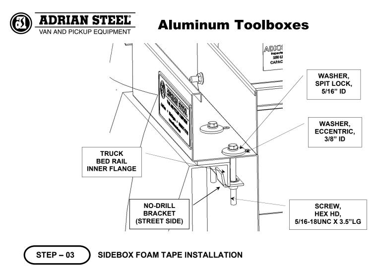
Cut supplied foam tape into (2) 20 inch long sections. Apply tape to the side box (street and curb side). Position foam tape approximately centered on side box flange as shown in detail views below. After foam tape has been applied, slit the tape in all four slots to allow inserting of no-drill bracket fasteners.
