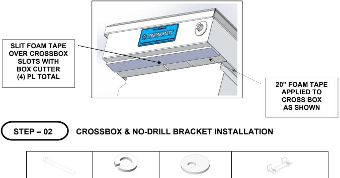
21660-0 **FAS0433 FAS0098** WASHER, NO-DRILL BRACKET SCREW, HEX HD, WASHER. SPLIT ECCENTRIC, 5/16-18UNC X 3.5" LOCK, 5/16" ID 3/8" ID (4) REQ'D (4) REQ'D (4) REQ'D
