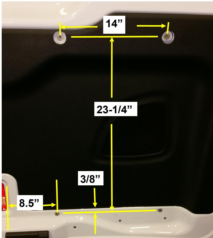
POSITION ASSEMBLY TO THE INSIDE OF THE REAR DOOR PANEL(S) ACCORDING TO PACKAGE LAYOUT INSTRUCTIONS. MARK AND DRILL CLEARANCE HOLES THROUGH THE DOOR PANEL FOR THE TWO (2) UPPER MOUNTING LOCATIONS AND DRILL AND SET FOUR (4) 1/4" PLUSNUTS USING DIMENSIONS SHOWN
