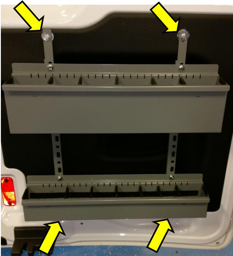
POSITION ASSEMBLY TO THE INSIDE OF THE REAR DOOR PANEL AND ATTACH USING TWO (2) FAS0018 SCREWS FOR THE BOTTOM ATTACHMENT AS SHOWN.
