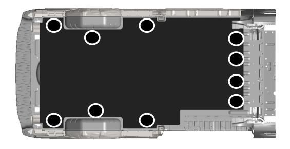
**Step 03** Drill and set plusnuts (FAS0091) centered in the holes just drilled in the floor liner. **Step 04** Install spacers and fasteners as shown below. Use the spacer that allows the cup washer to sit inside the lip on the top of the spacer. This will vary between mounting points
