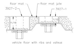
A PLUSNUT (RIVNUT) SETTING TOOL IS REQUIRED FOR PLUSNUT (RIVNUT) INSTALLATION. PLUS NUT SETTING TOOL CAN BE ORDERED THROUGH ADRIAN STEEL, OR USE AN AIR POWERED PLUSNUT SETTING GUN.
