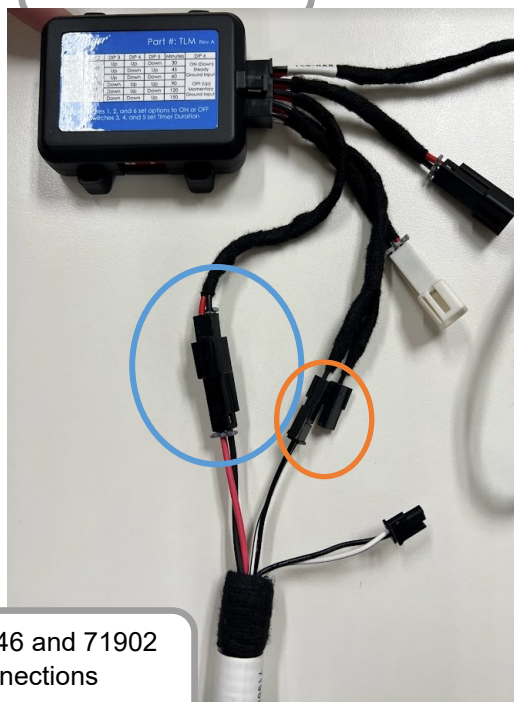
74546 fed through firewall, connected to TLM
