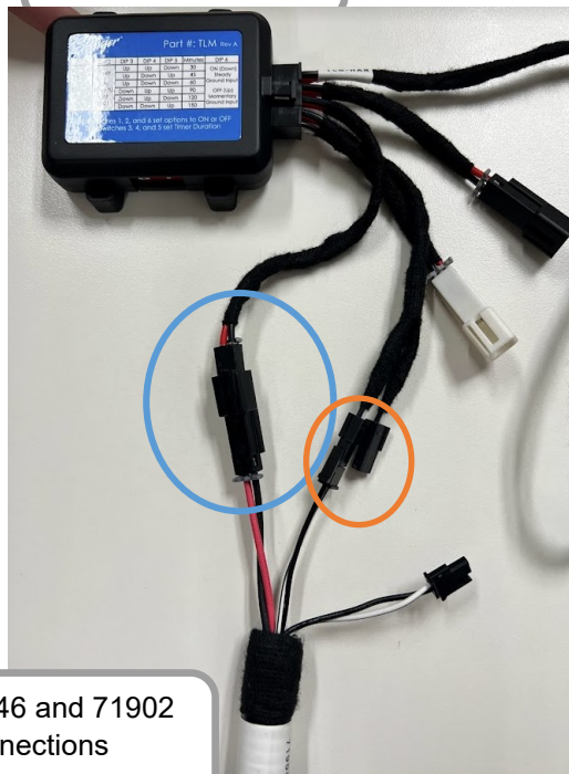
74546 fed through firewall, connected to TLM
