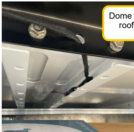
Dome light on roof bow
