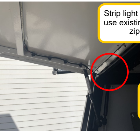
Leave extra wiring for opening the door
