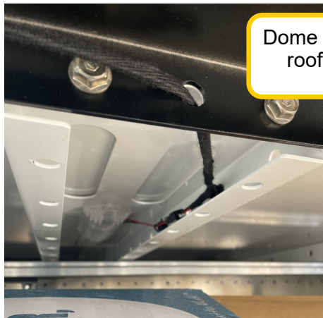
Dome light on roof bow
