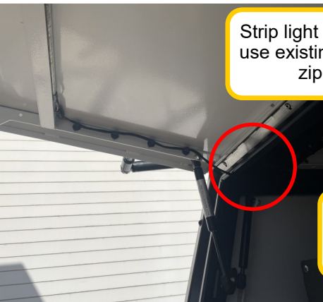
Leave extra wiring for opening the door
