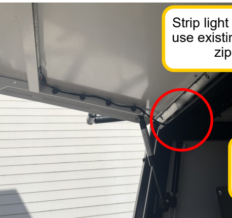
Leave extra wiring for opening the door
