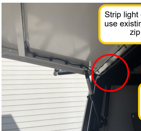
Leave extra wiring for opening the door
