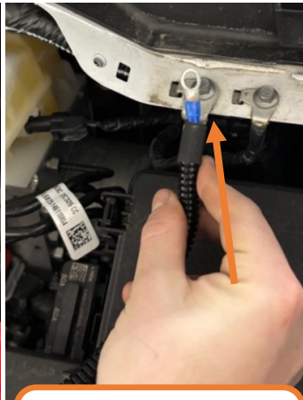
Negative stud [located near driver side firewall] - attach ring terminal
