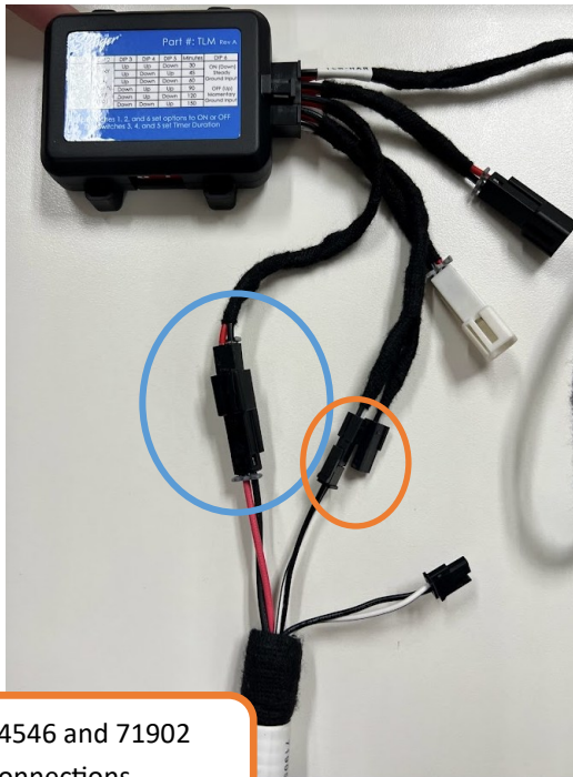
71904 fed through fire-wall, connected to TLM
