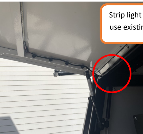
Leave extra wiring for opening the door
