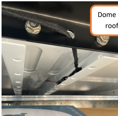
Dome light on roof bow
