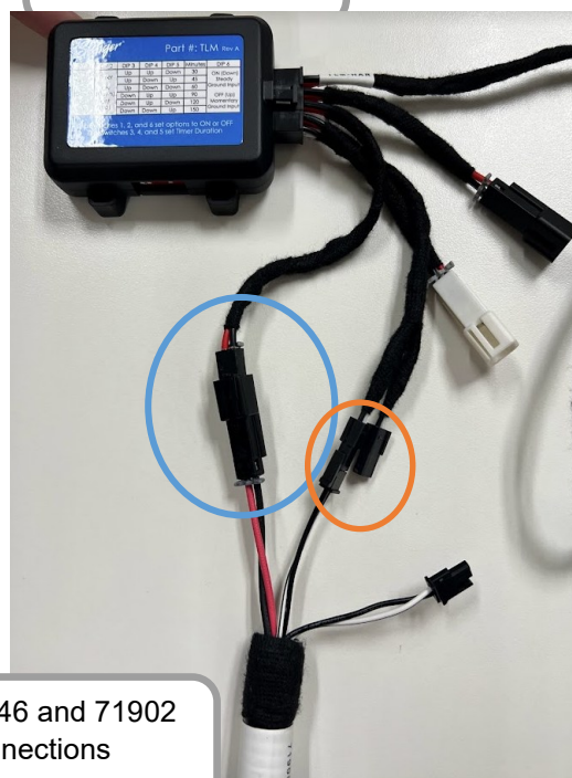
74546 fed through firewall, connected to TLM
