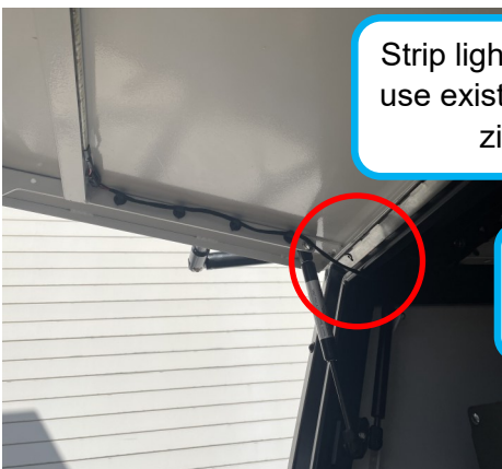
Leave extra wiring for opening the door
