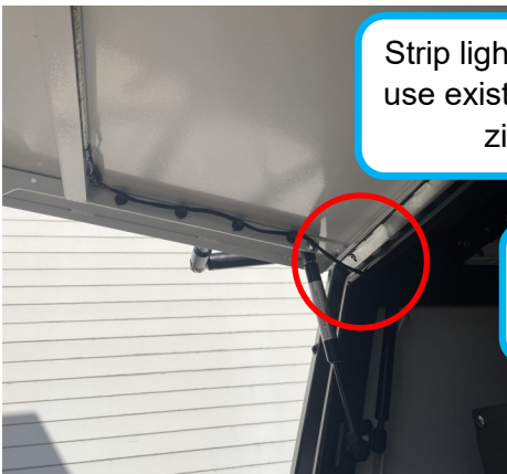
Leave extra wiring for opening the door
