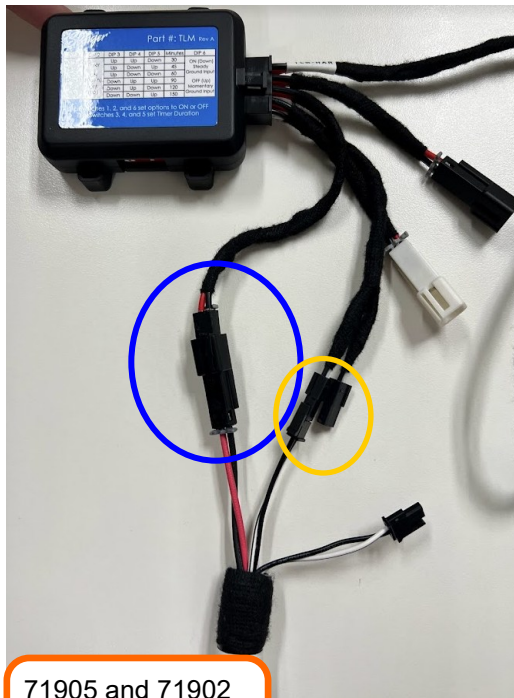
71903 fed through firewall, connected to TLM
