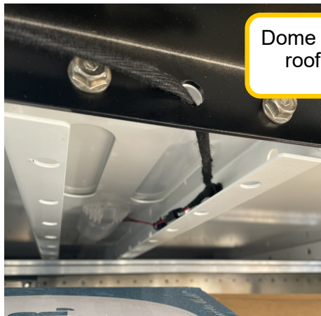
Dome light on roof bow
