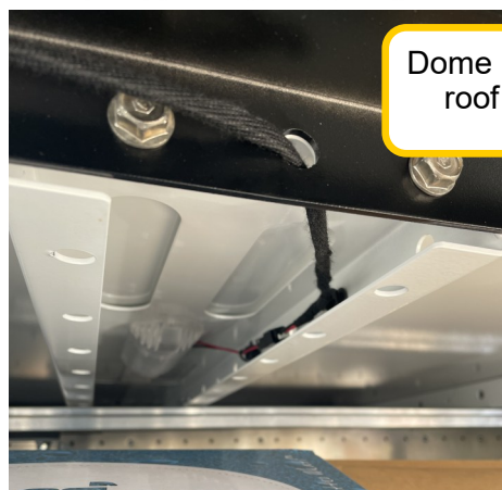
Dome light on roof bow
