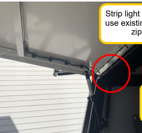
Leave extra wiring for opening the door
