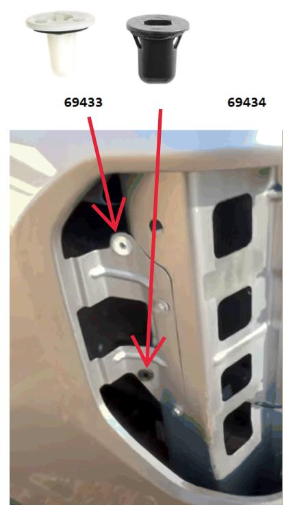
Single Use Clips - replace these after removing the taillight
