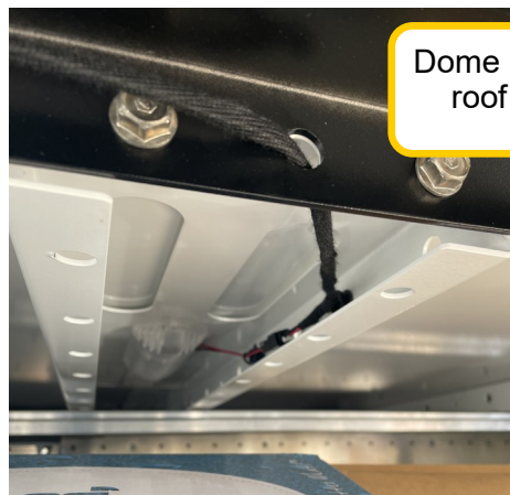
Dome light on roof bow
