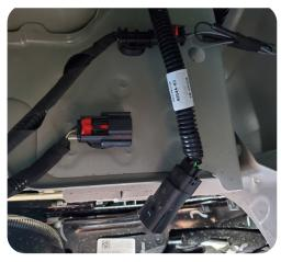
**STEP 3:**Install the P-BUA-COLORADO-23 harness between the two OEM connectors
