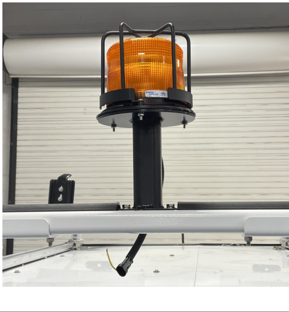
Beacon: Middle Of Rear Cross Bow
