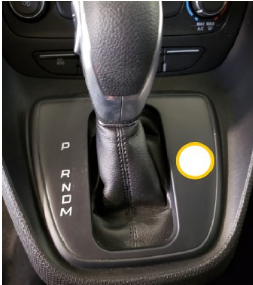
Switch placement: On Shift Column Panel
