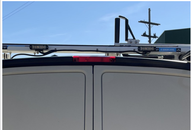
Front / Rear Strobes: Middle Of Cross Bows
