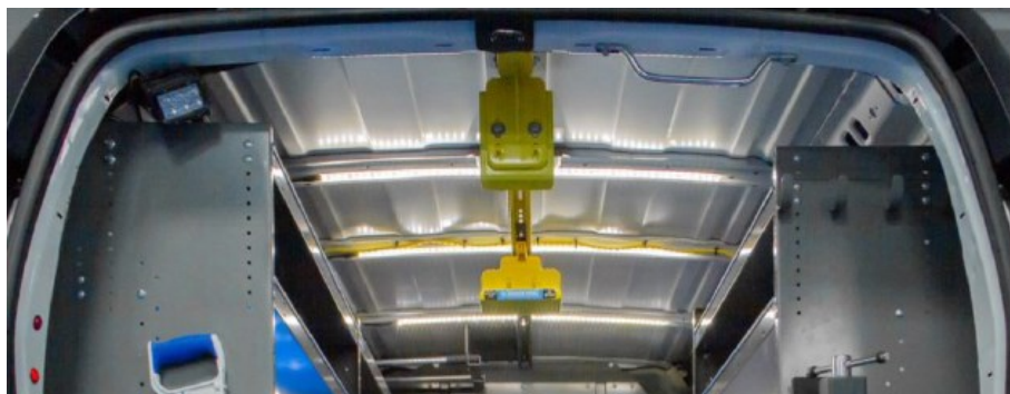
LED Light Strips Installed on Roof Bows
