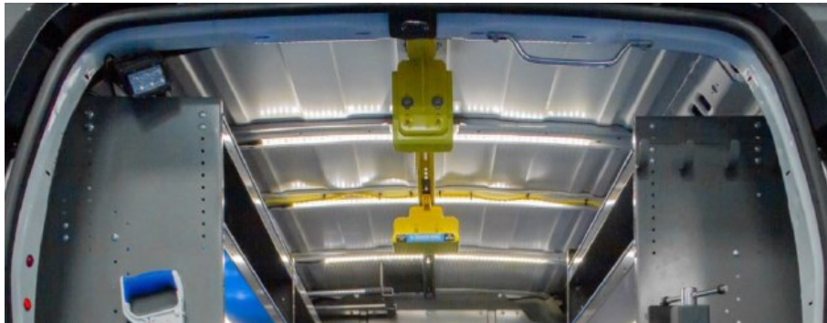
LED Light Strips Installed on Roof Bows
