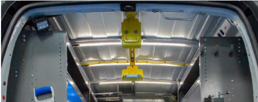
LED Light Strips Installed on Roof Bows
