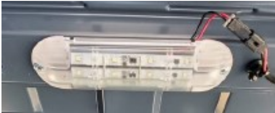
LED Dome Light Installed on the Roof Bow
