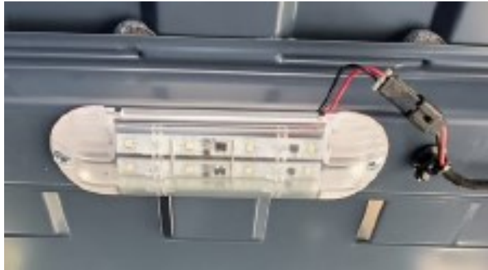
LED Dome Light Installed on Roof Bow
