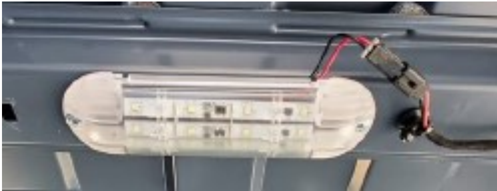
LED Dome Light Installed on Roof Bow
