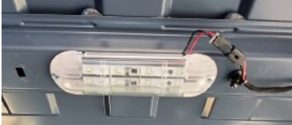
LED Dome Light Installed on Roof Bow
